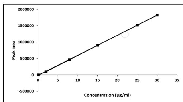
**Fig. 5.** Calibration curve for determination of CSOL in the pure form at  $\lambda_{\text{max}} = 230$  nm using the proposed method.
