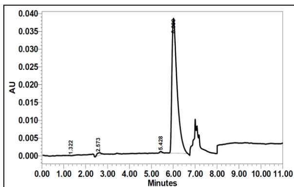
**Fig. 7.** HPLC chromatogram of Hexitol<sup>®</sup> solution showing a peak of 10.00 µg/ml of CHX at a timed wavelength of 265, 260 & 230 nm.
