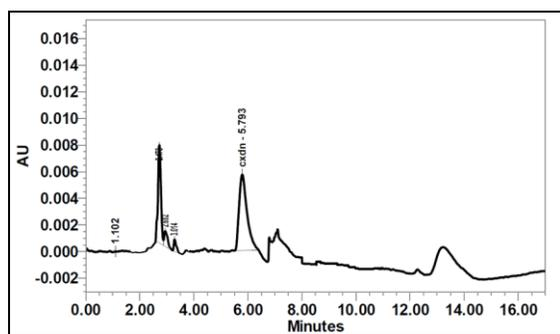
**Fig. 9.** HPLC chromatogram of saliva spiked with 2.00  $\mu\text{g/mL}$  CHX at a timed wavelength of 265, 260 & 230 nm.
