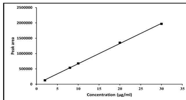
Fig. 4. Calibration curve for determination of CHX in pure form at  $\lambda_{\text{max}} = 260$  nm using the proposed method.
