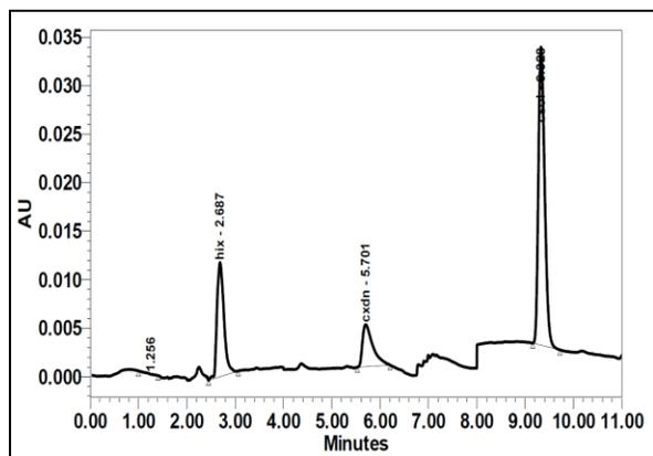
**Fig. 6.** HPLC chromatogram of Cyteal<sup>®</sup> douche showing simultaneous separation of 2.50 µg/mL HEX, 12.50 µg/mL CHX & 7.50 µg/mL CSOL at a timed wavelength of 265, 260 & 230 nm; respectively.
