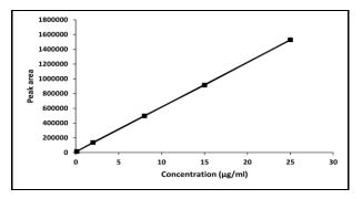
Fig. 3. Calibration curve for determination of HEX in pure form at  $\lambda_{max}$ = 265 nm using the proposed method.
