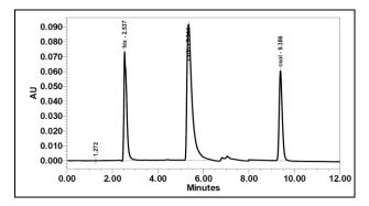
Fig. 2. HPLC chromatogram of the pure drugs showing simultaneous separation of HEX, CHX & CSOL (10.00  $\mu$ g/mL each) at a timed wavelength of 265, 260 & 230 nm; respectively.
