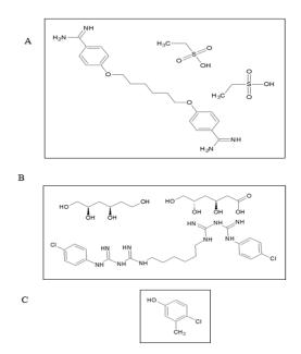
**Fig. 1.** The chemical structure of a) HEX b) CHX c) CSOL. (The structures were drawn by a Chem-Sketch program).
