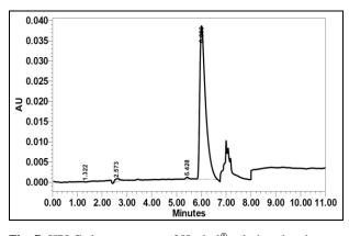
Fig. 7. HPLC chromatogram of Hexitol<sup>®</sup> solution showing a peak of 10.00  $\mu$ g/ml of CHX at a timed wavelength of 265, 260 & 230 nm.
