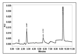
**Fig. 6.** HPLC chromatogram of Cyteal<sup>®</sup> douche showing simultaneous separation of 2.50  $\mu$ g/mL HEX, 12.50  $\mu$ g/mL CHX & 7.50  $\mu$ g/mL CSOL at a timed wavelength of 265, 260 & 230 nm; respectively.
