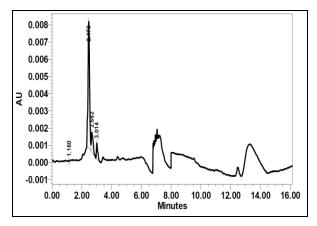
Fig. 8. HPLC chromatogram of blank saliva at a timed wavelength of 265, 260 & 230 nm.
