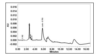
Fig. 9. HPLC chromatogram of saliva spiked with 2.00  $\mu$ g/mL CHX at a timed wavelength of 265, 260 & 230 nm.
