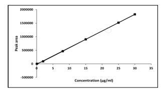
Fig. 5. Calibration curve for determination of CSOL in the pure form at  $\lambda_{max}$ = 230 nm using the proposed method.
