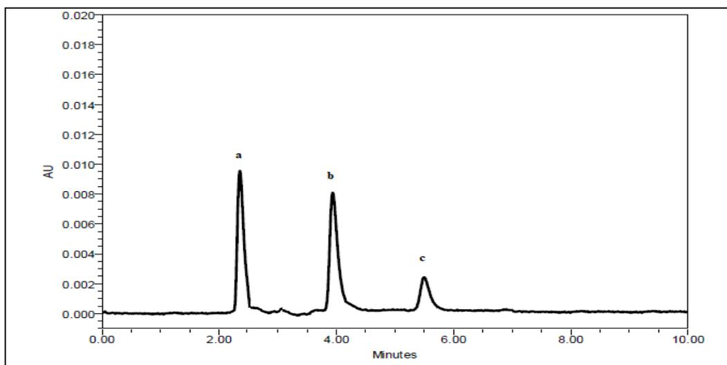
**Fig. 2.** HPLC Chromatogram of (a) DCF (600 ngmL<sup>-1</sup>), (b) CBZ (600 ngmL<sup>-1</sup>) and (c) TCS (600 ngmL<sup>-1</sup>) using UV detection at 283 nm
